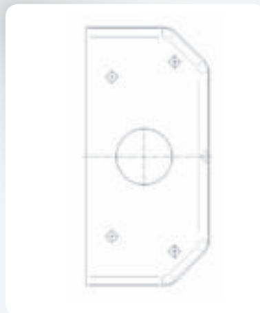
Version with two holes for mounting SNCD..MH1
