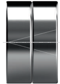
Outer raceway markings for paired bearings
