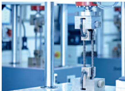
More than 15 pulser are available for testing dynamic fatigue strength according to different testing methods
