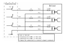
Figure 4: Connection to PNP signal (common-cathode)
