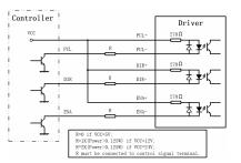
Figure 3: Connections to open-collector signal (common-anode)
