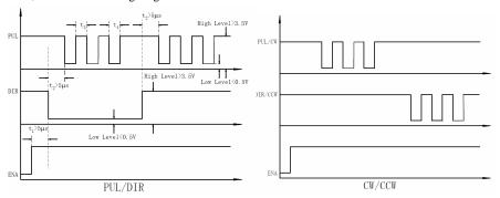
Figure 11: Sequence chart of control signals
